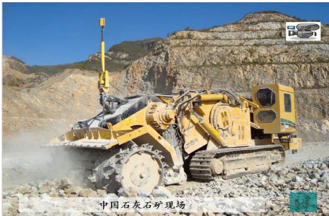
Direct Mining with Horizon King Continuous Surface Miner
