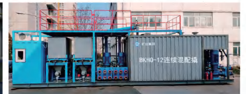
石油压裂液混配撬 / 车 Full-automatic oil fracturing fluid mixing skid / vehicle
