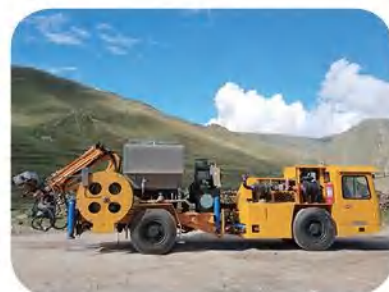
智能地下乳化炸药现场混装车 Intelligent underground emulsion charging truck
