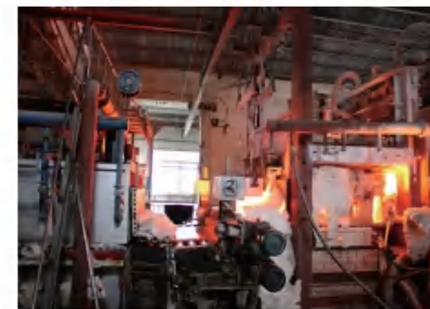
冶炼危险固废渣玻璃化处置 Vitrification of hazardous smelting solid wastes
