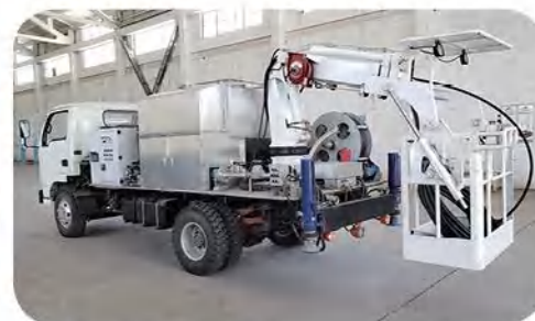
地下乳化炸药现场混装车 Underground emulsion charging truck
