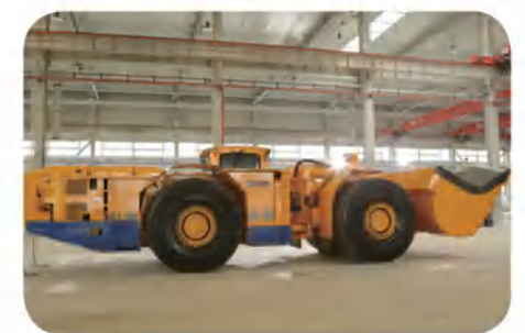
混合动力铲运机 Hybrid LHD of model AHCY514, a innovative product of biggest LHD weigh with 14 tons load
