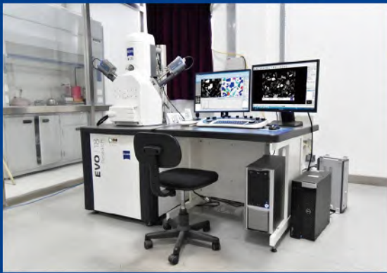
Fig.1 BPMA system based on ZEISS EVO18 SEM and Bruker QUANTAX 200 EDS at the BGRIMM Technology Group (Figure provided by Prof. M.X. Jia)
