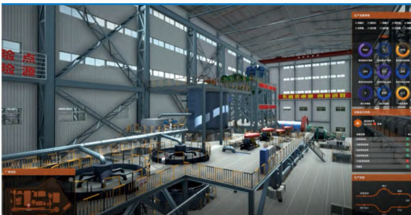
Digital twin and 3D visualization interface of grinding expert system
