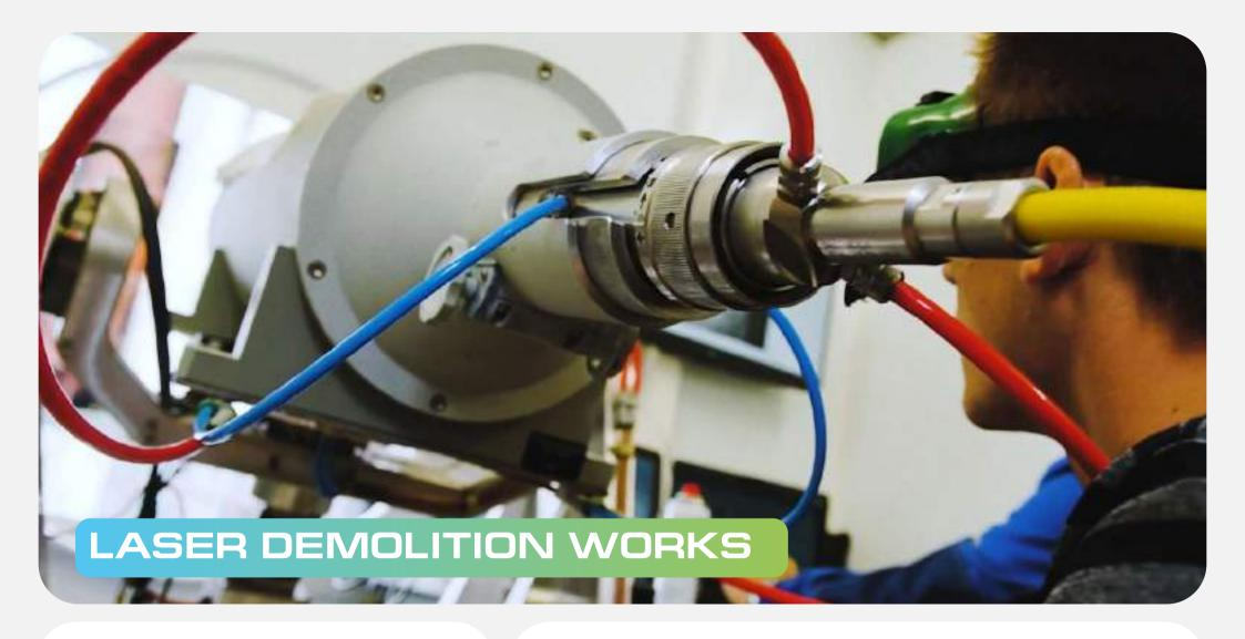
A method of destroying and removing building materials using high-intensity laser beams.
