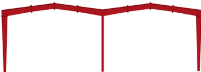
**MULTIGABLE** buildings have a roof with 2 or more gables, vertical sidewalls and vertical end walls. Interior bay frames are rigid frames.
