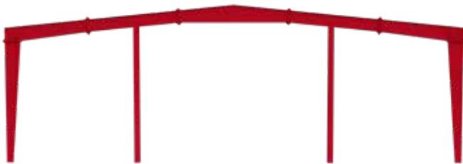
**MULTISPAN MS-2** buildings have a gable roof with vertical sidewalls and end walls. Interior bay frames are rigid frames. The designation MS-2 implies two interior columns, and so on.
