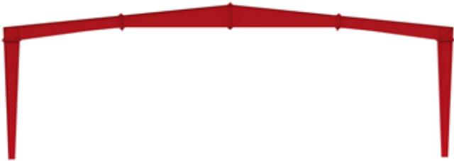
**CLEAR SPAN** buildings have a gable roof with vertical sidewalls and end walls. Interior bay frames are clear span rigid frames (without interior columns).
