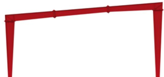
**MONO SLOPE** is a building with the sloping roof in one plane. The slope is from one wall to the opposite wall.
