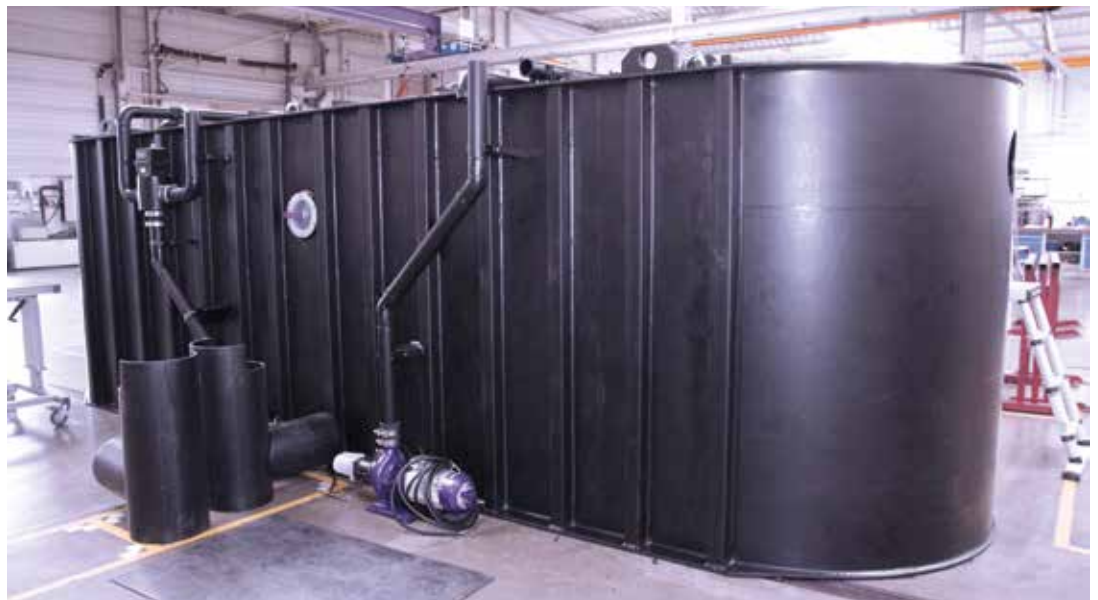
Surpassing themselves for success: the company not only created the largest grease separators in the history of KESSEL during the project, but also the largest grease separator in the world with a nominal size of 50 (max. 50l/s). (Source: KESSEL AG)
