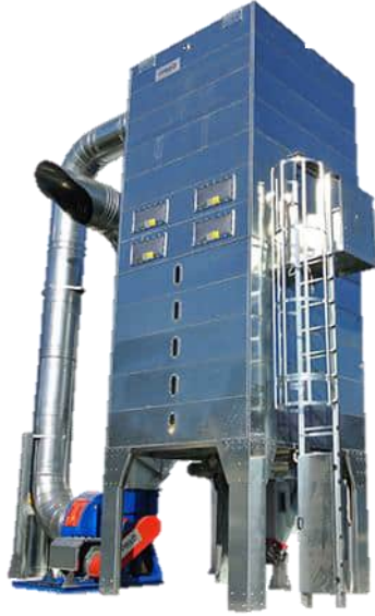
COIMA MVD Mini-Silo Baghouse Dust Collectors with Mechanical Shaker Cleaning System
