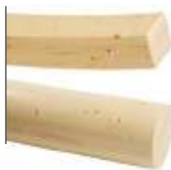
Curved spruce with small lamellas
