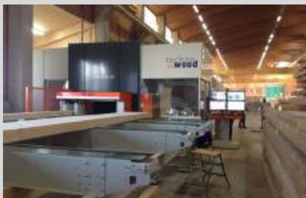
High speed CNC machine for straight beam
