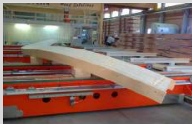
New generation CNC machine for free form project element
