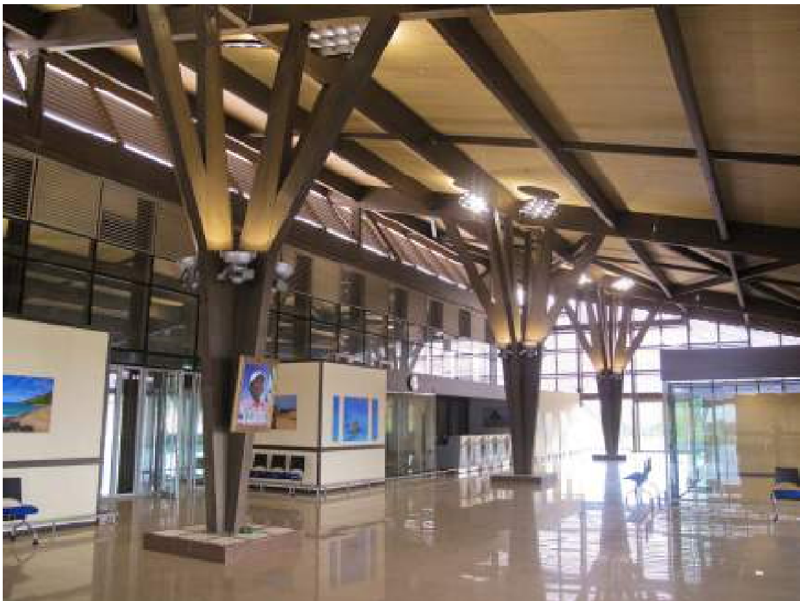
Annobon island (Equatorial Guinea) Airport Terminal Glulam structure with Résix® connections Sapisol® roofing with special acoustic profile
