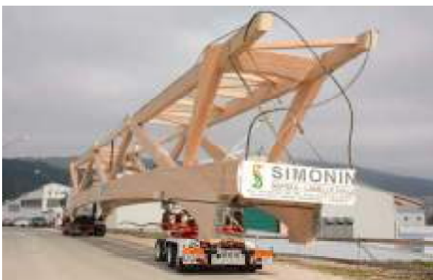
Logistics : road/sea/air Transport of 40m long bridge
