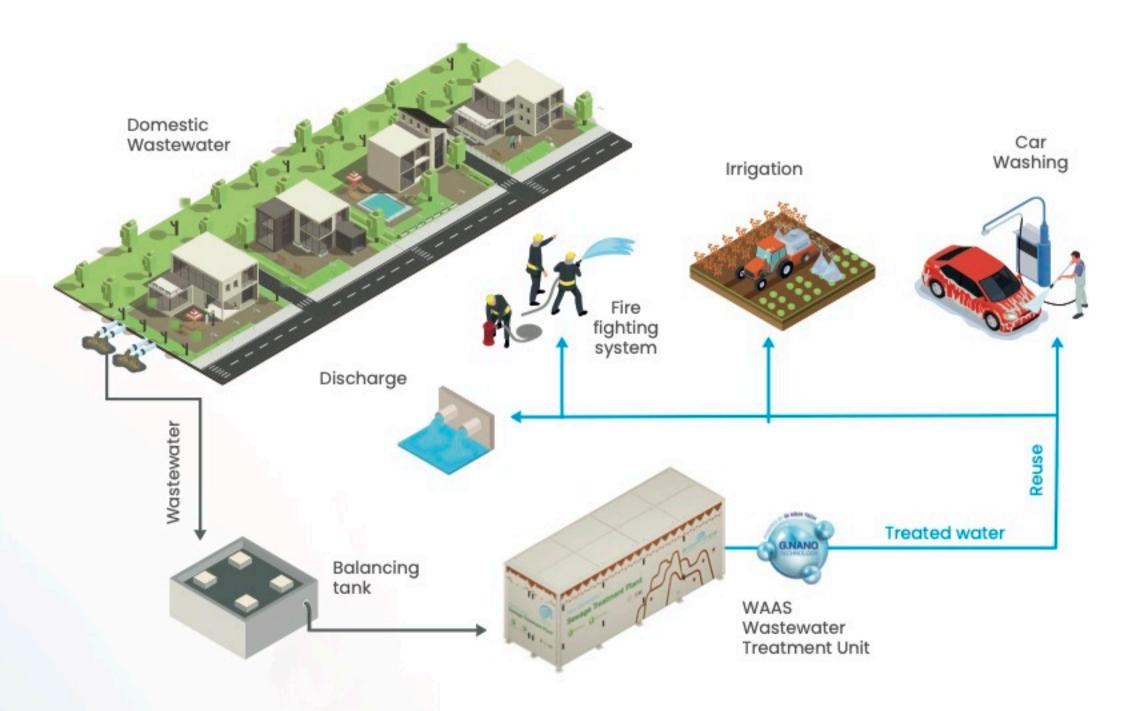
WAAS deployed an 18 m² containerized treatment unit that met every requirement. The system produced crystal-clear water reused entirely on-site for landscaping and cooling. Operating silently and consuming just 0.2 kWh/m³, it demonstrated how even the most sensitive environments can achieve sustainable, high-performance wastewater treatment — without compromise
