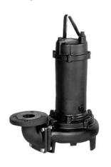
Flow upto 2.2 m3/min Head upto 20 m Power 1.5 kW to 7.5 kW Material of Construction : CI/CI/SS
