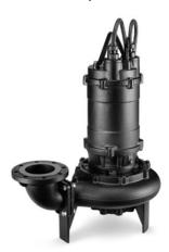
Flow upto 2.8 m3/min Head upto 29.4 m Power 2.2 kW to 22 kW Material of Construction : CI/CI/SS
