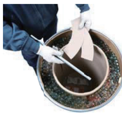
Removing the steel bar and pads
